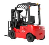
The EFL201 is a reliable all-rounder forklift for both indoor and outdoor tasks, thanks to its high ground clearance, big tyres and water resistance.
